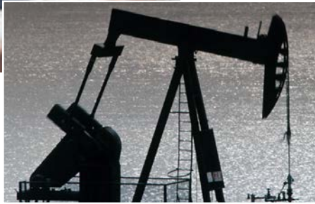
A pump jack is used for extracting petroleum from an oil well.
