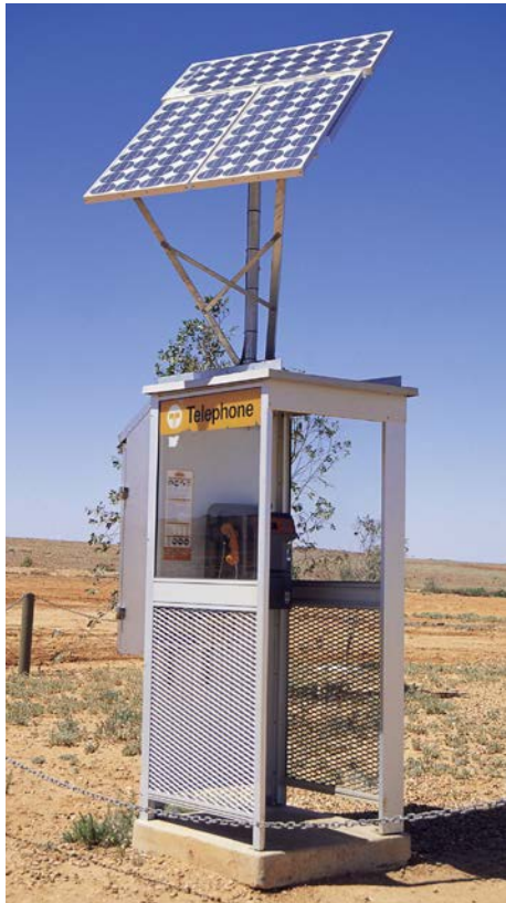
A solar panel is used to provide energy to this phone booth.
